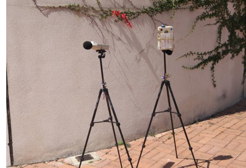
Air quality monitoring is conducted by Environmental Consultant every 6 days at the nearby ASR.
